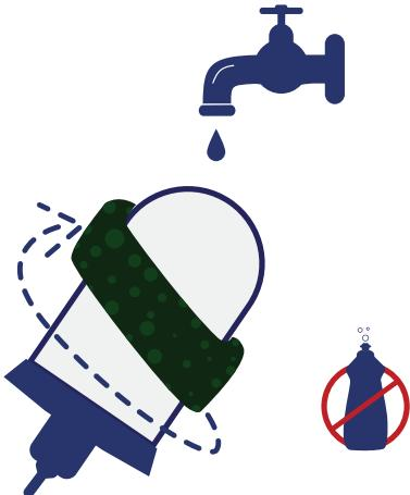
1. When the filter is clogged, scrub using a sponge under running water.
