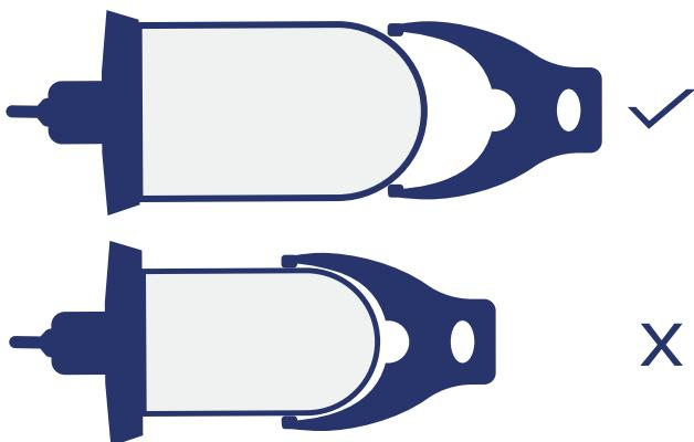
Can filter up to 7000 liter and needs to be replaced when diameter is less than 5 cm.
