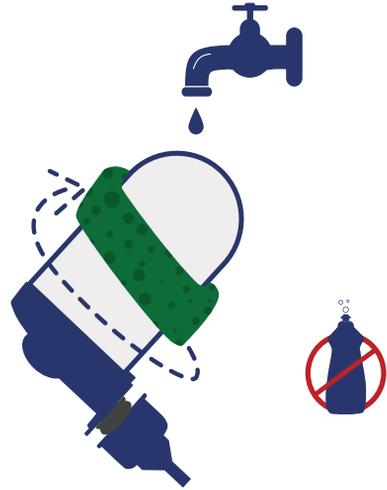
1. When the filter is clogged, scrub using a sponge under running water.
