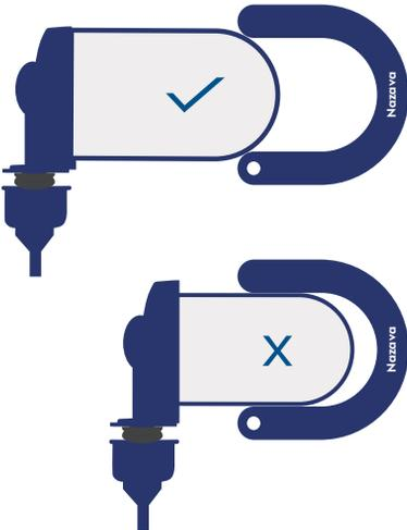
Can filter up to 7000 liters and needs to be replaced when diameter is less than 5 cm.
