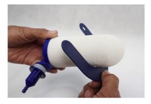
When the ceramic filter element becomes less than 5 cm the filter element needs to be replaced. The old filter element needs to be disposed safely.
