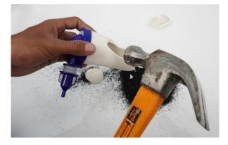
iii. Separate the ceramic (white), activated carbon (black) from the plastic (blue) cap
