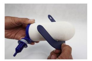
When the ceramic filter element becomes less than 5 cm the filter element needs to be replaced. The old filter element needs to be disposed safely.
