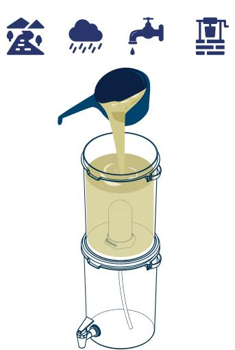
2. Pour RIVER WATER, RAIN WATER, TAP WATER or WELL WATER into the upper container until full.
