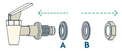
2. Remove the nut and seal B attached to the tap. Leave seal A on the tap.
