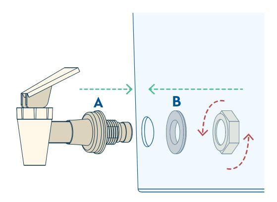
3. Install the tap and seal A from the outside of the lower container into the hole.
