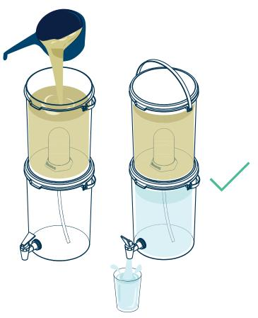
4. Refill the upper container. Wait for the water to filter into the lower container.
