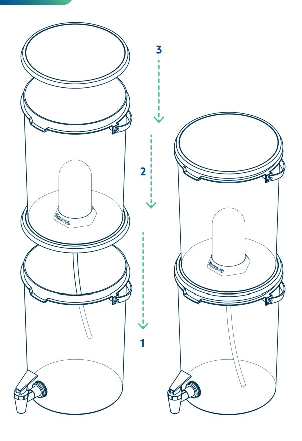
6. Place the upper container with the ceramic filter on the lower container.
