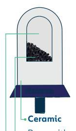
Pores with a size of 0.4 micron block bacteria.
