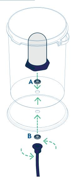
5. Install the ceramic filter and seal A into the hole inside the upper container.
