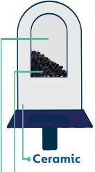
Pores with a size of 0.4 micron block bacteria.
