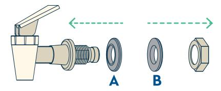
2. Remove the nut and seal B attached to the tap. Leave seal A on the tap.
