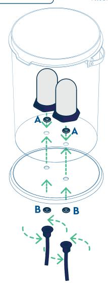
5. Install the ceramic filter and seal A into the hole inside the upper container.
